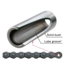
Tsubaki's general use G7-EX roller chains utilize a seamless solid bush thanks to our unique production technology. (Available for RS40 – RS240 chains.) The high precision solid bush utilizes special lube grooves (LG) to increase lubricant retention and give the chain twice the wear life.
