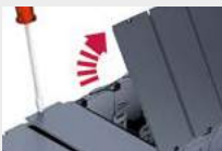
Simply unlock cover with a screwdriver
