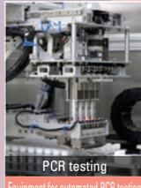
Equipment for automated PCR testing
