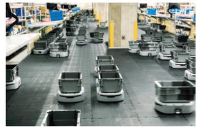
T-Carry System, a handling and sorting system using small AGVs (2020)
